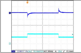
Figure 5: Output Voltage Response to Step-Change in Load Current (50 %-75 % -50 % of Iout(max);  $dI/dt = 0.1 A/\mu s$ . Load cap: 1  $\mu F$  ceramic cap. Ch 1: Vout, Ch 2: Iout (5 A/div).
