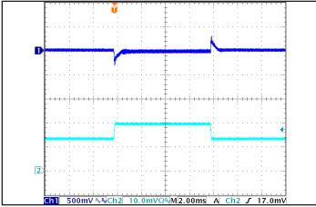
Figure 5: Output Voltage Response to Step-Change in Load Current (50 % -75 % -50 % of Iout(max); dI/dt = 0.1 A/ $\mu$ s. Load cap: 15  $\mu$ F tantalum cap and 1  $\mu$ F ceramic cap. Ch 1: Vout, Ch 2: Iout (20 A/div).
