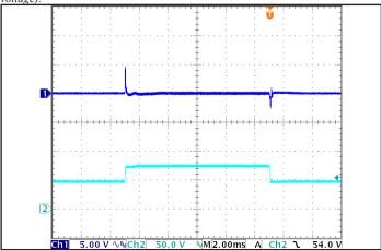
Figure 6: Output Voltage Response to Step-Change in Input Voltage (500 V/ms), at Max. load current. Load cap: 100  $\mu$ F electrolytic cap and 1  $\mu$ F ceramic cap. Ch 1: Vout, Ch 2: Vin.
