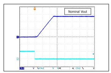
Common Figure 1: Startup Waveform (typical). Input voltage pre-applied, ON/ OFF Pin on Ch 2. Output voltage normalized.
