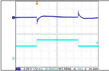
Figure 5: Output Voltage Response to Step-Change in Load Current (50 % -75 % -50 % of Iout(max); dI/dt = 0.1 A/ $\mu$ s. Load cap: 15  $\mu$ F tantalum cap and 1  $\mu$ F ceramic cap. Ch 1: Vout, Ch 2: Iout (5 A/div).
