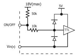
Figure B: Internal ON/OFF Pin Circuitry
