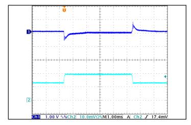
Figure 5: Output Voltage Response to Step-Change in Load Current (50 % -75 % -50 % of Iout(max); dI/dt = 0.1 A/ $\mu$ s. Load cap: 15  $\mu$ F tantalum cap and 1  $\mu$ F ceramic cap. Ch 1: Vout, Ch 2: Iout(10 A/div).
