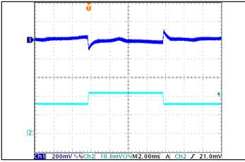
Figure 5: Output Voltage Response to Step-Change in Load Current (50 %-75 %-50 % of Iout(max); dI/dt = 0.1 A/µs). Load cap: 15 µF tantalum cap and 1 µF ceramic cap. Ch 1: Vout, Ch 2: Iout (20 A/div).
