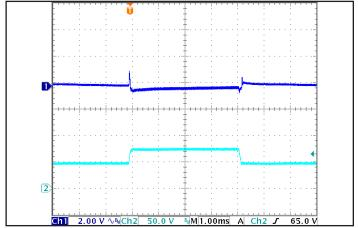
Figure 6: Output Voltage Response to Step-Change in Input Voltage (500 V/ms), at Max. load current. Load cap:  $100\mu F$  electrolytic cap and  $1\mu F$  ceramic cap. Ch 1: Vout, Ch 2: Vin.
